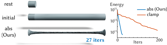
Fig. 7. We stress test our abs projection strategy under large stretching (11x) with high Poisson’s ratio \nu = 0.4999 . Here we create the initial deformation by moving the rightmost vertices of a cylinder by a factor of 10x.
