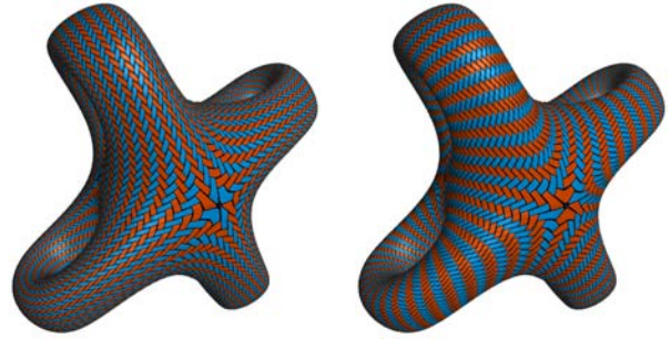
Figure 15: Diagonal twill-weaving patterns on a quad mesh obtained by remeshing a (16, 4, 4) regular mesh.
