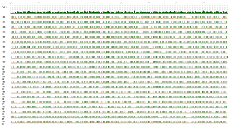
Figure 9: A Threadscope log of Chan's algorithm, with 22 threads and 2^{24} points.
