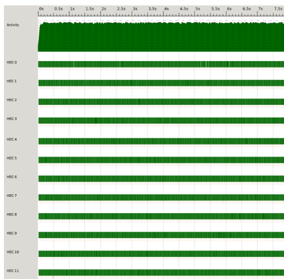
Figure 7: A zoomed out picture of the load balancing for 1000 particles across 12 threads.
