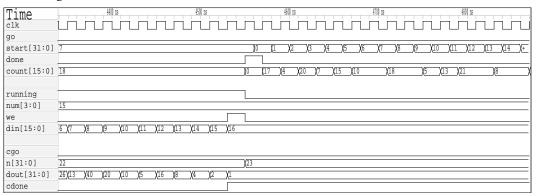
After *we* is asserted for the highest RAM address (15, set by *RAM\_WORDS*), *running* turns off and *done* pulses once. This tells the testbench to feed 0, 1, 2, ... into *start* and the number of iterations for each value is read out on *count*. For example, *start* = 0 produces a 17 on *count*, corresponding to n = 7, and *start* = 11 produces a 21, corresponding to n = 7 + 11 = 18. Running the *Vrange* simulator directly prints out these iteration counts:
