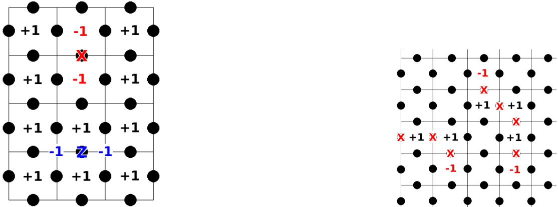
Figure 3: (left) Single X error flips the sign of both adjacent Z stabilizers because of anti-commutation relation, i.e. for a state |\psi\rangle stabilized by Z_a Z_b Z_c Z_d , error X_c yields X_c |\psi\rangle = X_c (Z_a Z_b Z_c Z_d |\psi\rangle) = -Z_a Z_b Z_c Z_d (X_c |\psi\rangle) . Similarly, a Z error flips the sign of the adjacent X stabilizers (only affected X stabilizers indicated). (right) Two chain of X errors, only affected stabilizers shown. Note one chain connects to the smooth boundary and only changes the sign of a single stabilizer. Intermediate Z stabilizers remain in +1 eigenstates. Z stabilizers at end of the error chains become negative.
