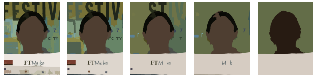
Figure 6: Depth map completion. Starting with an over-segmented image (left), the segments are iteratively merged based on color, texture and depth using a greedy algorithm. Note how the number of segments N_s decreases with the iterations (left to right).
