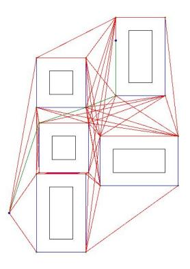
Figure 1: Visibility graph on grown obstacles shown, with Dijkstra's shortest path in green.
