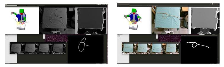
Above are the screens that come up. The top left is the osg viewer, where the training rope points red and the testing rope points are blue. The trajectories are red and green for old and new trajectories, respectively. The program requires you to step through the simulation before it executes on the robot. In the bottom window, we see the nearest neighbors ranked. And we also see the original image from the kinect, greyed out as well as the masked result.
