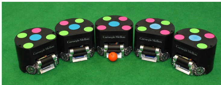
Figure 3 Vision targets arranged in unique patterns, detected by an overhead RGB camera, can enable more robust robot localization. These are RoboCup Small Size League robots.
