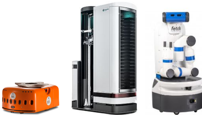
Figure 1 From left to right: Kiva, TORU, Fetch. Each platform supports varying levels of autonomous navigation between points given a 2D map of the environment.
