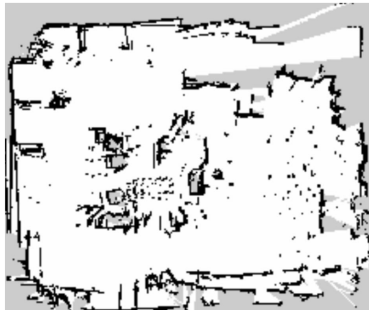
Figure 2 A 2D obstacle map of the testing environment.
