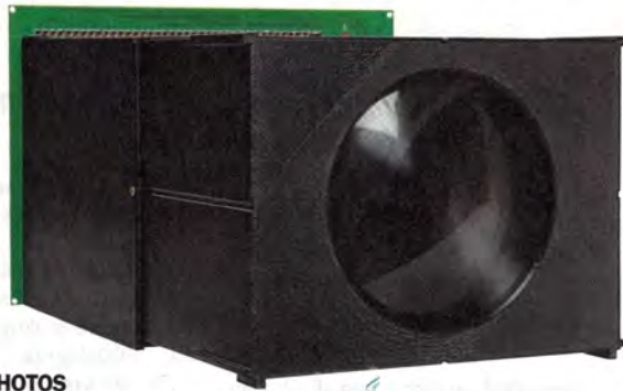
PHOTOS FOREVER With enough light, the prototype Eternal Camera (above right) can continuously power itself thanks to an image sensor (left) that doubles as a solar panel.
