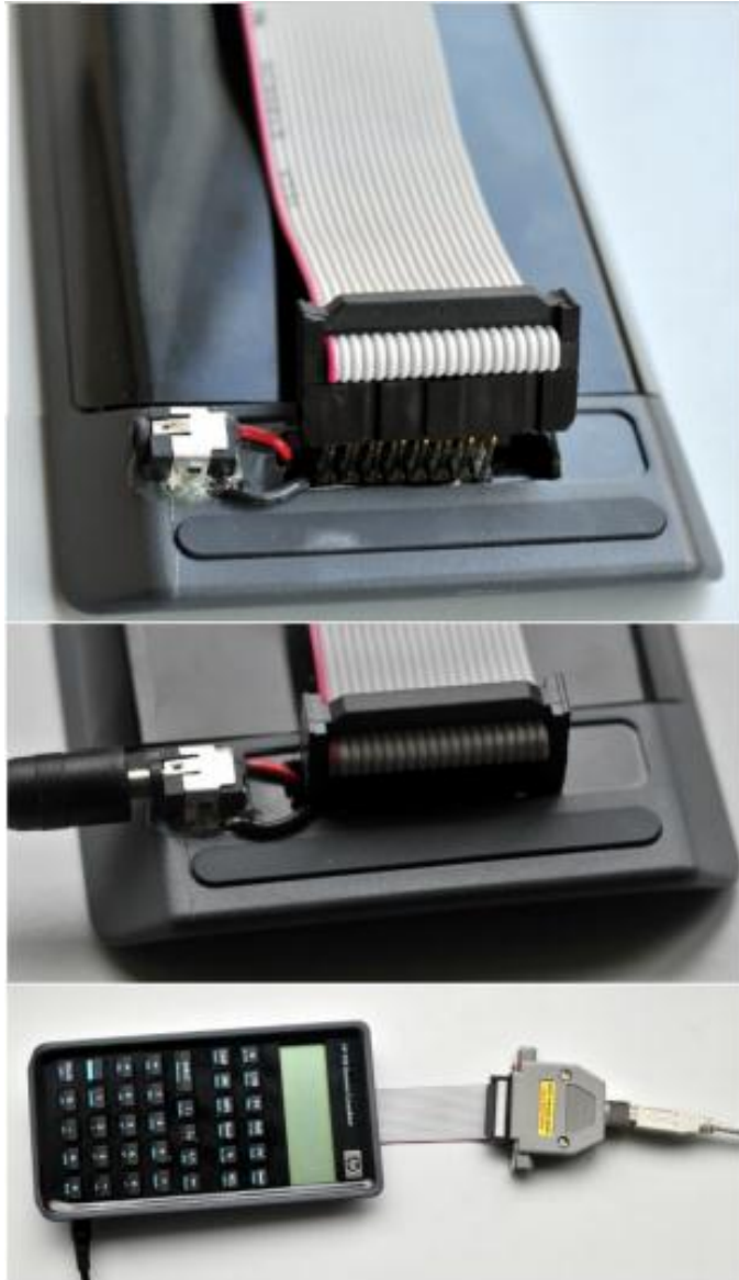
Figure 2: The Calculator's JTAG connector (Courtesy of Professor Edwards)
